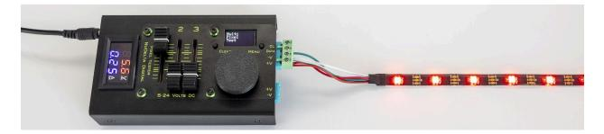
LED tape connected using the 5.5 millimeter DC input connector.
