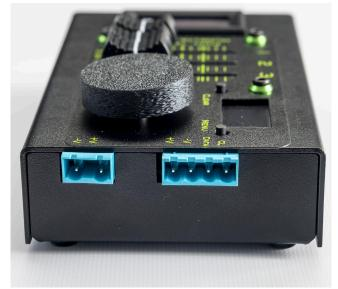
Removable Phoenix-style connectors on the right side. The connector on the left, marked with V+ and V-, is for power input. The connector on the right is for the LEDs.
