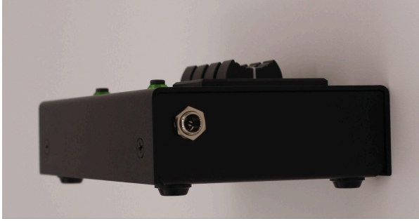
5.5 millimeter input connector on left side
